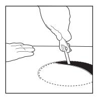
b. Draw a circle on the tile using the compass tool and a pencil. Cut the circle out of the ceiling tile.
